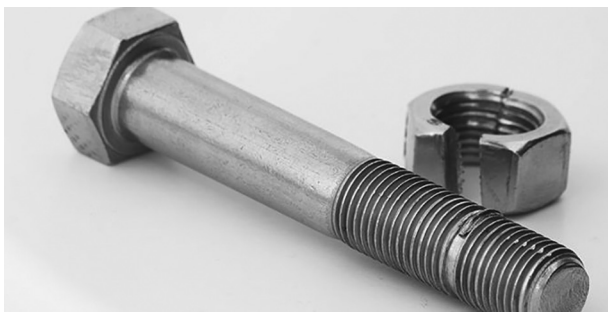
Fig. 2-1. A bolt and nut that have suffered from galling.
